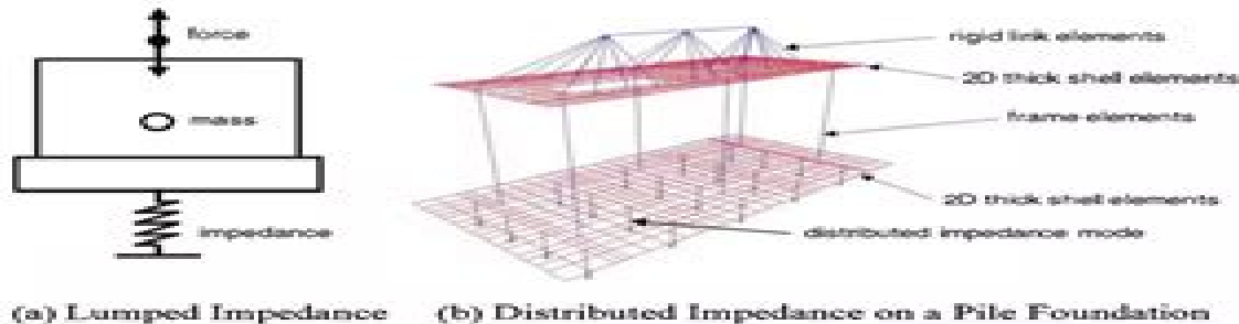
Fig. 6.3.2b—Lumped and distributed soil impedance.
