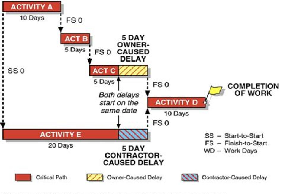
The two 5 WD delays are literal, concurrent delays because they both started on the same day and are of equal duration.
