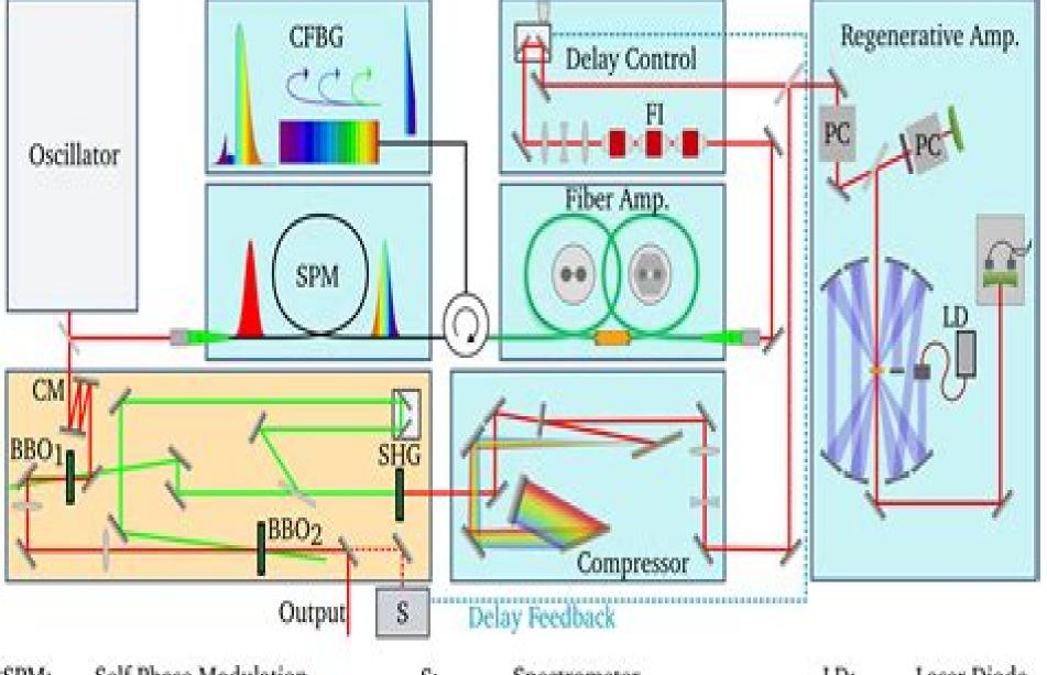
SPM: Self-Phase Modulation LD: Laser Diode S: Spectrometer Beta-Barium Borate CFBG: Chirped Fiber Bragg Grating BBO:
