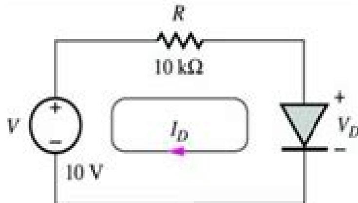
$V$  and  $R$  may represent the Thévenin equivalent of a more complex 2-terminal network. The objective of diode circuit analysis is to find the quiescent operating point for the diode.
