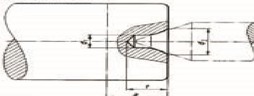
Designation of a radius form 60° centre hole without protective chamber (R1), with diameter  $d_1 = 8$  mm and diameter  $d_2 = 8,5$  mm:
