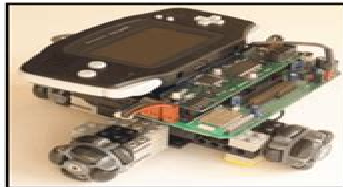
Photo 1 —Lego is an excellent medium for implementing robots such as the four-wheeled HUMR. The Gameboy Advance acts as the controller and provides 32-bit RISC processing performance, a color LCD, and sound.
