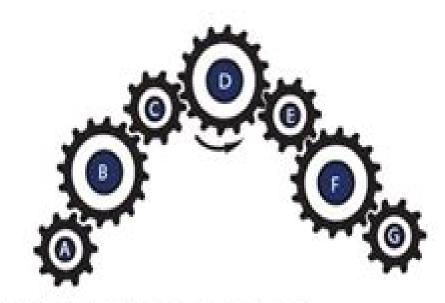
If gear A is turning at a rate of 700 turns per second, at what rate will gear G be turning?
