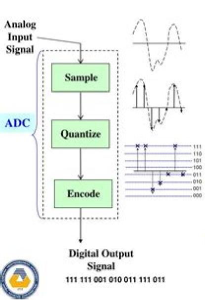
➤ The Analog-to-digital Converter (ADC) performs three functions:
