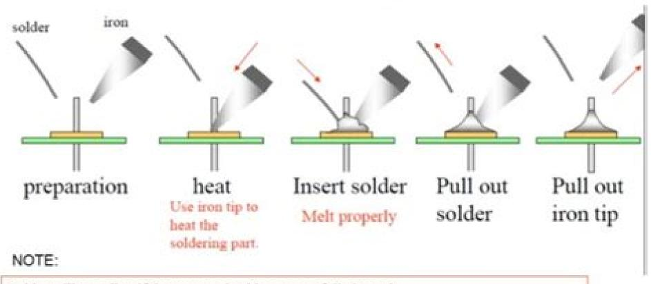
Solder will not alloy if the parts and solder are not fully heated.
