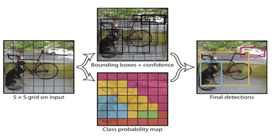
**Figure 2: The Model.** Our system models detection as a regression problem. It divides the image into an  $S \times S$  grid and for each grid cell predicts B bounding boxes, confidence for those boxes, and C class probabilities. These predictions are encoded as an  $S \times S \times (B*5+C)$  tensor.
