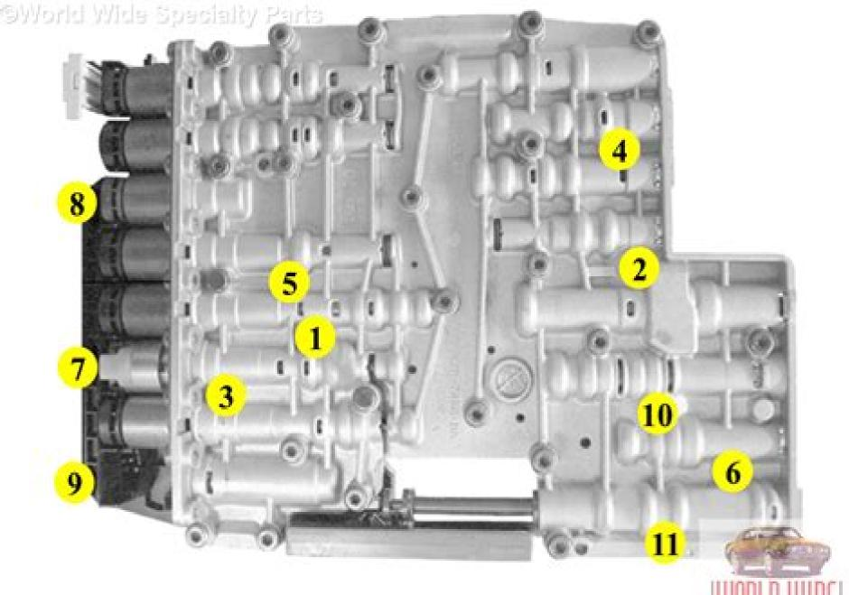
Torque Valve Body Bolts in Sequence Shown To 53 Inch It
