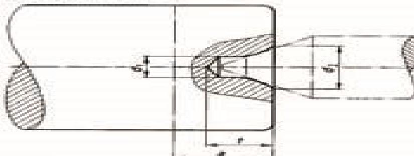
Designation of a radius form 60° centre hole without protective chamber (R1), with diameter  $d_1 = 8$  mm and diameter  $d_2 = 8,5$  mm:
