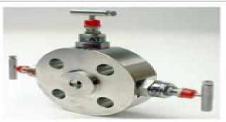
Gauge block monoflange valves work in conjunction with a pre-installed primary isolate valve. They provide compact instrument double block and bleed valving. This range is also available in both single block and single block and bleed configurations.
