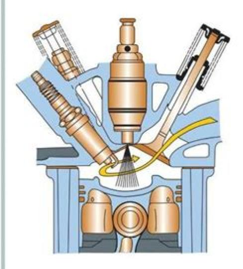
FIGURE 20–1 A gasoline directinjection system injects fuel under high pressure directly into the combustion chamber.
