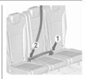
Remove lower latch plate from retainer and click it into left-hand buckle (1) at the centre seat. Guide the upper latch plate with the belt over the lap area and the shoulder (do not twist) and click into right-hand buckle (2) at centre seat.
