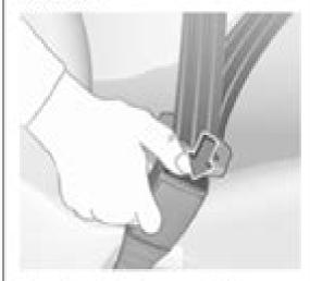
To release belt, press red button on belt buckle.
