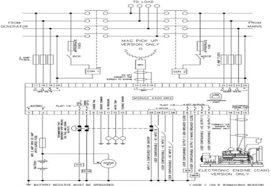
\*\* MOTE 3. IT IS RECOMMENDED THAT THE GENERATOR AND MAINS SMITCHING DEVICES ARE MECHANICALLY AND ELECTRICALLY INTERLOCKED.
