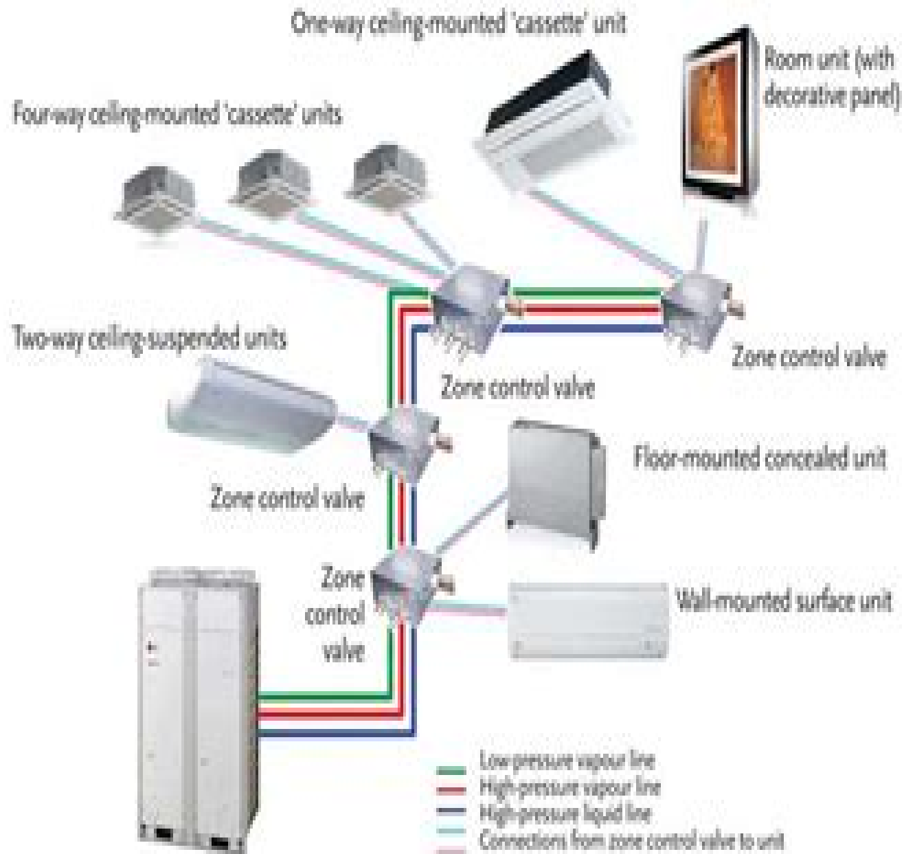
Figure 1: An example three-pipe VRF system
