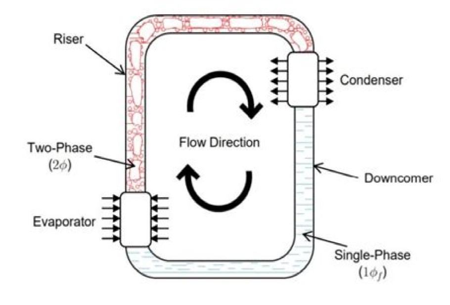
FIGURE 1: Schematic diagram of a closed-loop thermosyphon.
