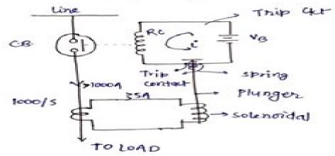
every equipment on the P.S. is connected through ce a typical cht Breaker consist of two fixed contact of one moving contact. The moving contact is held with fixed contact. Then energy flows from line to the local the system is initially designed in such a way that for normal operating current the magnetizing force produce by the sameterial could solenoised
