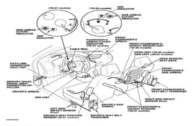
Fig. 1: Locating SRS Components
