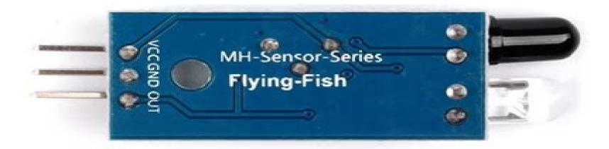
IR Infrared Obstacle Avoidance Sensor Module
