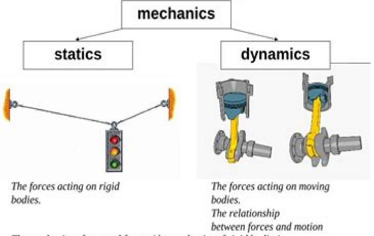
The mechanics of external forces (the mechanics of rigid bodies).
