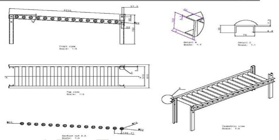
Fig. 2. Details of gravity roller conveyor
