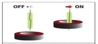
Fig. 1 LEFT - liquid level low, reed switch open. RIGHT - liquid level high, switch closed.
