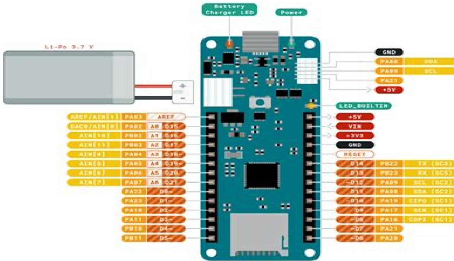
**Ground** **Internal Pin** **Digital Pin** **Microcontroller's Port**
