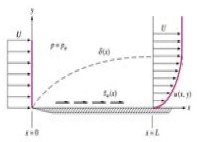
We consider only steady two-dimensional incompressible viscous flow with the x direction along the wall and y normal to the wall as shown in the figure. The complete equations of motion consist of continuity and the x- and y-momentum relations:
