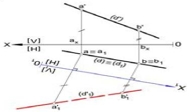
In order to determine the true length of the segment (AB), it is necessary that it has a certain position relative to one of a projection planes, so that it is projected on this plane, without deformation. In this case, we consider the segment (AB) parallel to a new vertical plane  $[V_1] \perp [H]$ , the new projection axis  $(O_2X_2)$  being parallel to the projection (ab). Hence, the line (D) (d, d') turned into a frontal line by changing of vertical plane.
