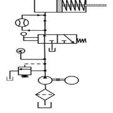
Figure 1.1 Control of a single-acting cylinder.
