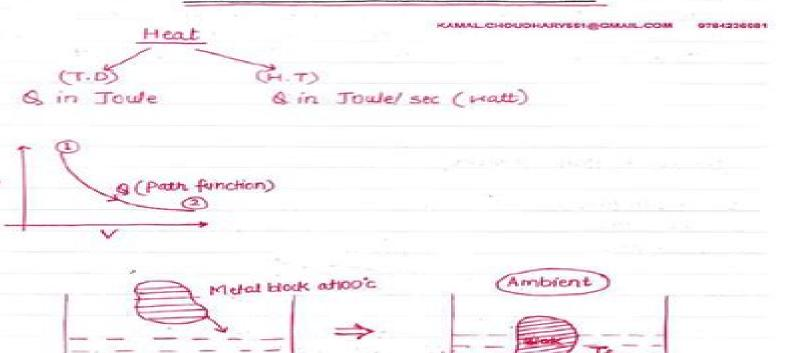
Heat lost by steel = Heat gained by water [energy balance equation]
