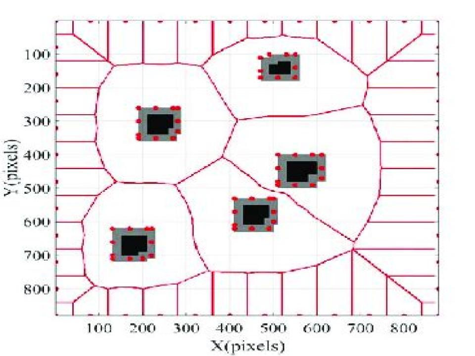
Robot Path Planning Using Geodesic And Straight Line Segments With Voronoi Diagrams Rsd Tr University Of Michigan Center For Research On Integrated Manufacturing Robot Systems Division
