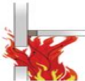
Perimeter Fire Containment System
