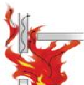
Unprotected Perimeter Joint
