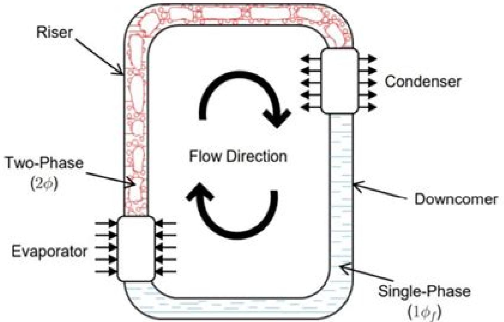
**FIGURE 1: Schematic diagram of a closed-loop thermosyphon.**
