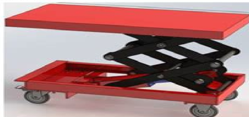
Fig.1. 3D modeling of hydraulic scissor lift
