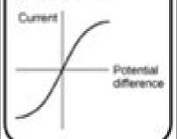
The current through a diade flows in one direction only. The diade has a very high resistance in the reverse direction.
