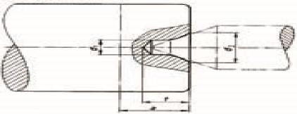
Designation of a radius form 60° centre hole without protective chamfer (R), with diameter  $d_1 = 4$  mm and diameter  $d_2 = 8.5$  mm:
