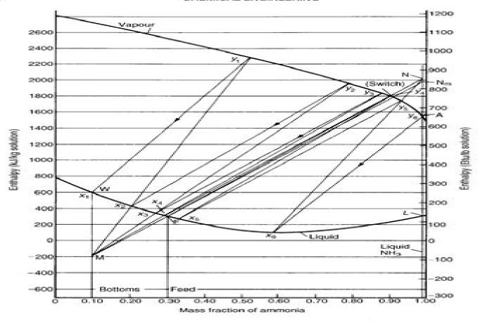
Figure 11.29. Enthalpy-composition diagram for ammonia-water at 1.0 MN/m2 pressure (Example 11.10)
